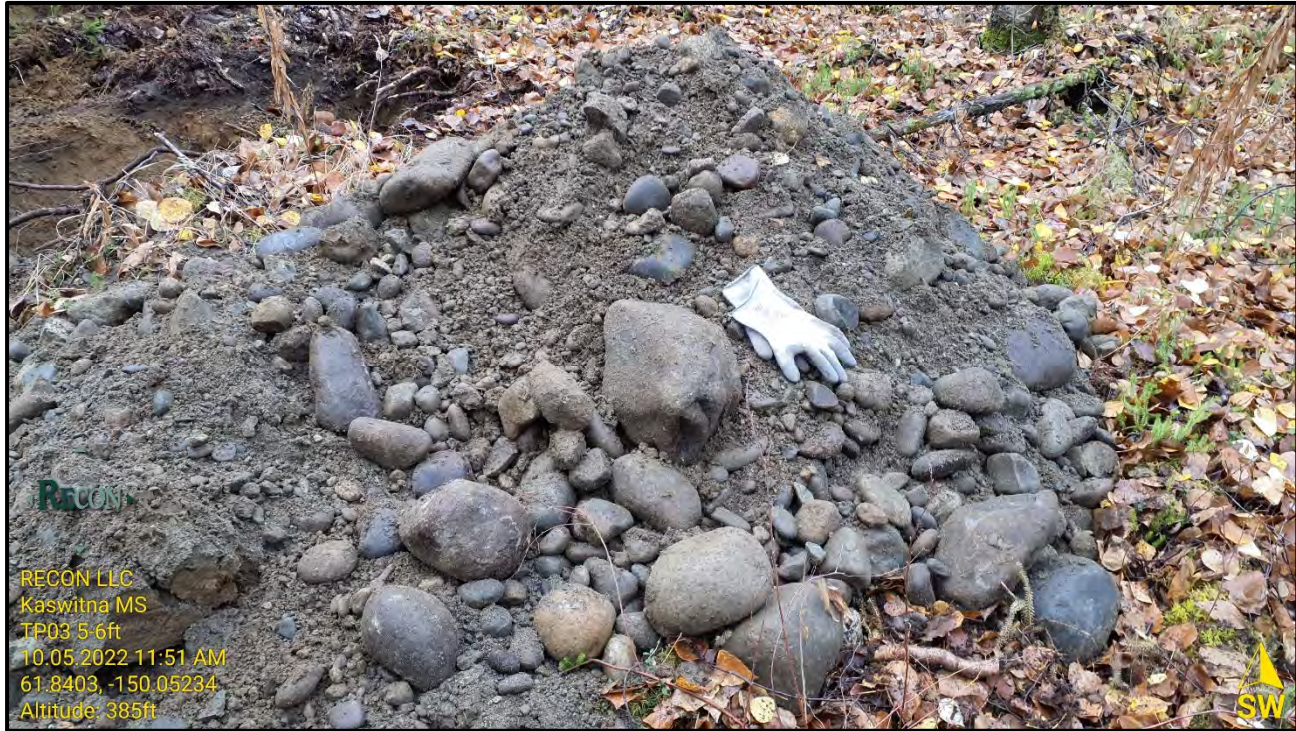
Figure 3. TP03 – Test pit excavated in relic river channel. Noticeably coarser material.
