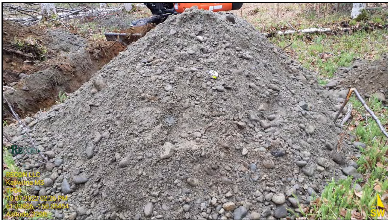
Figure 2. TP04 – Typical well-graded gravel with sand as observed in the top 10-feet of the relic terrace.
