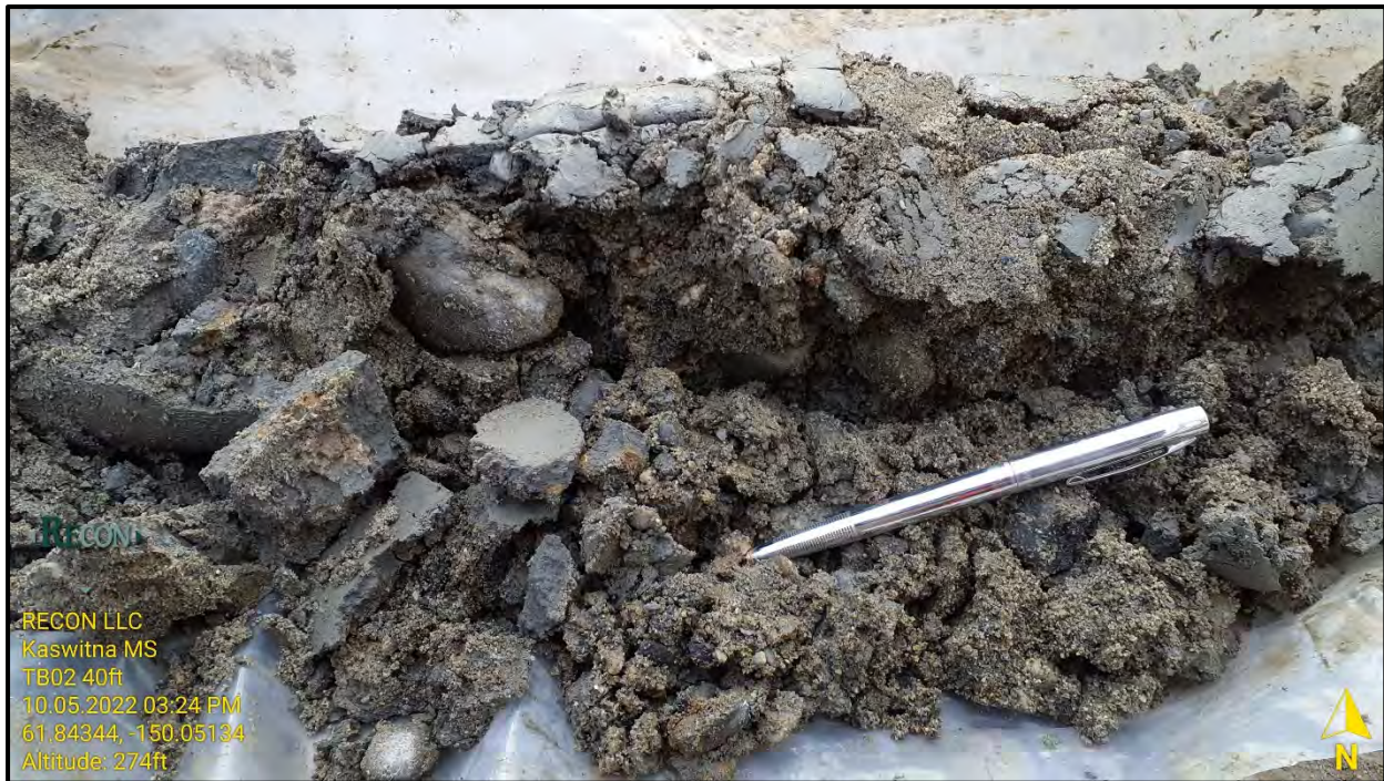
Figure 6. TB02 at 40' - Example of silty gravel with sand encountered in all test borings with est. 15% fines.
