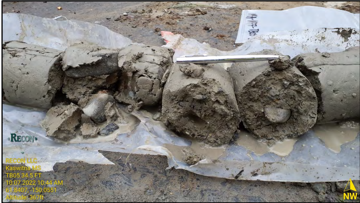
Figure 5. TB05 at 34.5' - Example of silty sand with gravel encountered in all test borings with ~32% fines.
