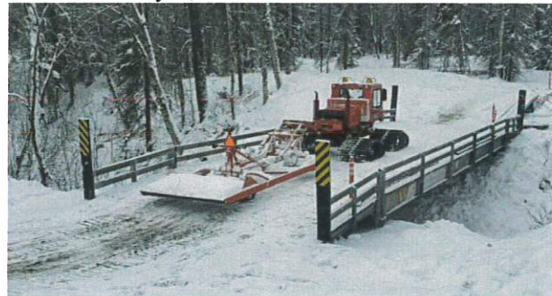
The Groomer Gully Bridge passes a load test with a Piston Bully trail groomer moving over the structure.
